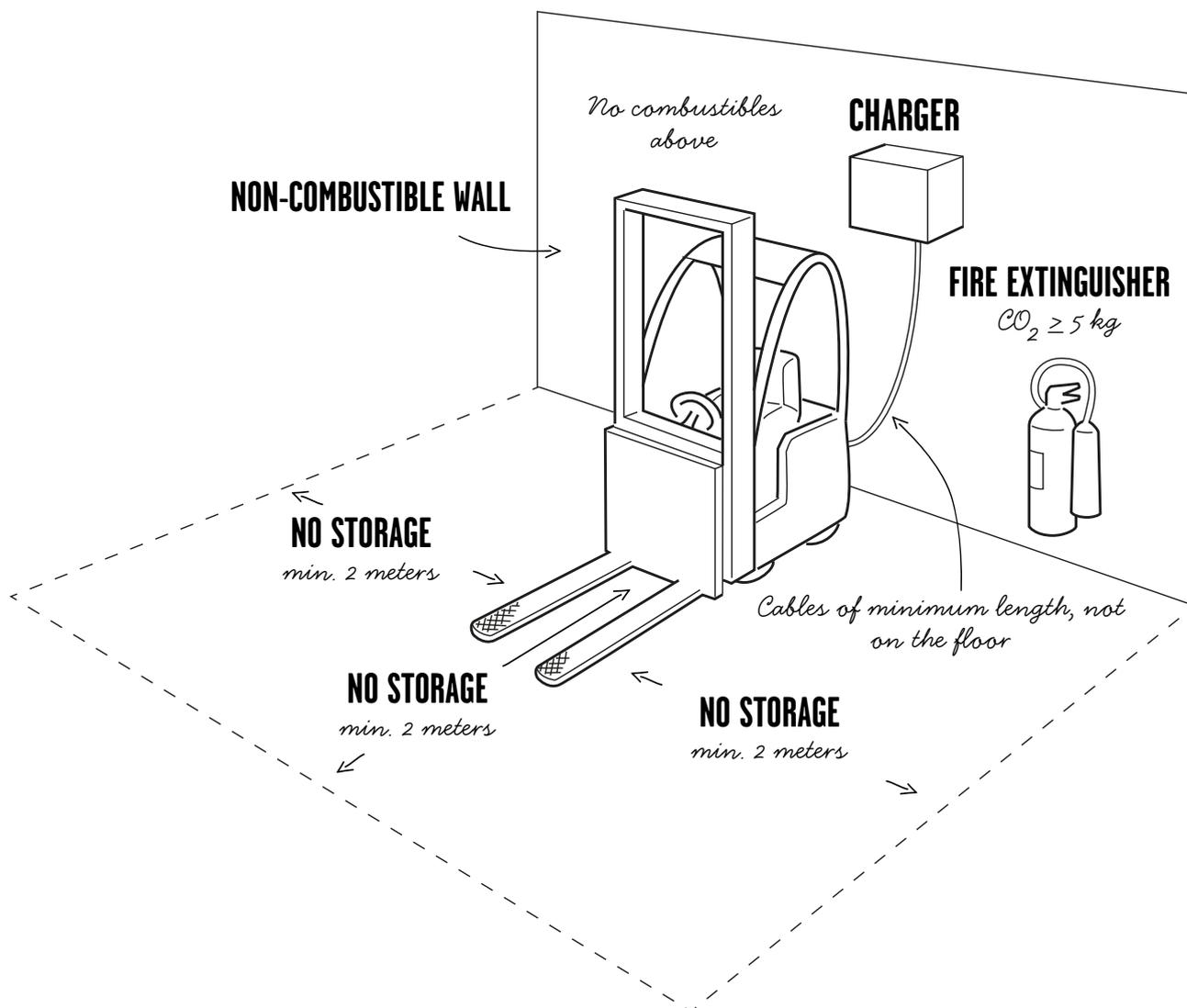
Batteries can be charged by an external unit, or by an internal charger, i.e. the equipment can be plugged-in to a normal electrical socket. In either case there is a risk of a fire starting. Because battery charging typically takes place in an out-of-the-way area or overnight, the fire may be able to develop without being detected. The fire will be able to grow quickly if there are combustible materials nearby.
